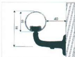
*SOCAVYL: Tubular handrail in rigid PVC.*
