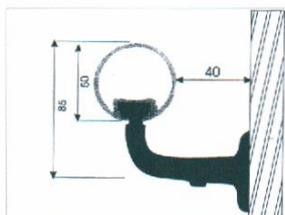
*SOCAVYL: Tubular handrail in rigid PVC.*
